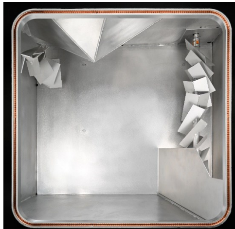
Fig. 1. Vertical stirrer inside The Wireless Connector®
