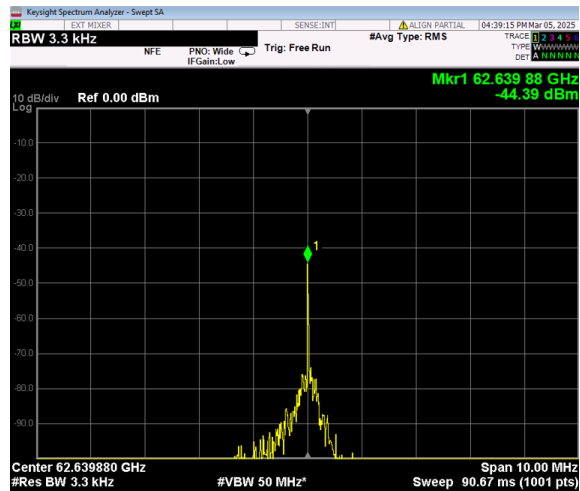
Fig. 10. Reduction in RBW causes reduction in peak power
